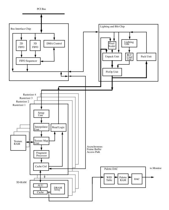
Each of the 3D-RAM chips has a 256-bit wide path between its cache and the DRAM array. The sixteen 3D-RAMS thus have a total bus width of 4096-bits. This provides a much greater bandwidth to memory than conventional designs.
